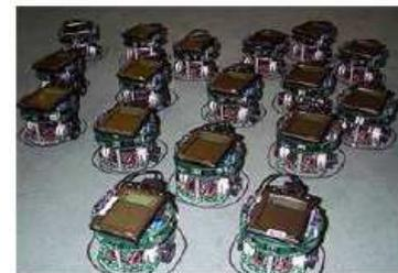
Fig. 2. A team of pherobots built for Darpa Software for Distributed Robotics program.
