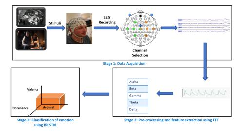
Fig. 6. Pipeline for human emotion recognition through EEG signals.
