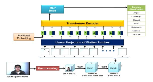
Fig. 4. Proposed vision transformer with convolution patches.
