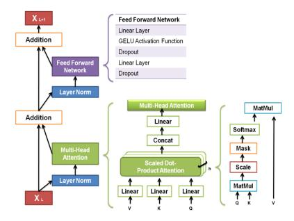
Fig. 5. Transformer encoder.
