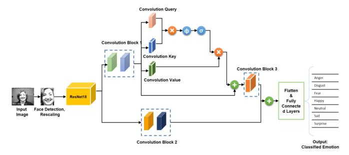
Fig. 2. FER through self-attention mechanism and transfer learning.
