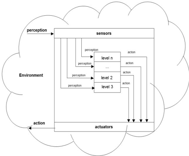
Fig. 18. A horizontal layered agent architecture (adapted from [21])
