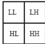
Fig. 2. (ii) Four sub-images after one-level wavelet decomposition
