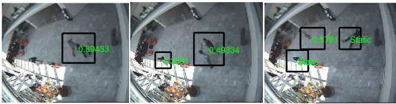
Figure 6. information content tracking, the three figures are respectively from Frame 220, 270, 350 in CAVIAR "Fight_OneManDown" database, the value in the rectangle correspond to the object information content
