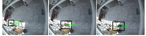
Figure 7. information content tracking, the three figures are respectively from Frame 570, 630, 690 in CAVIAR "Meet_Split_3rdGuy" database, the value in the rectangle correspond to the object information content
