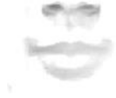
Figure 3. The subtracted image between source gray-scale I^{(0)} and the filtered image I_f . For observing conveniently, an image inverting transformation is employed.
