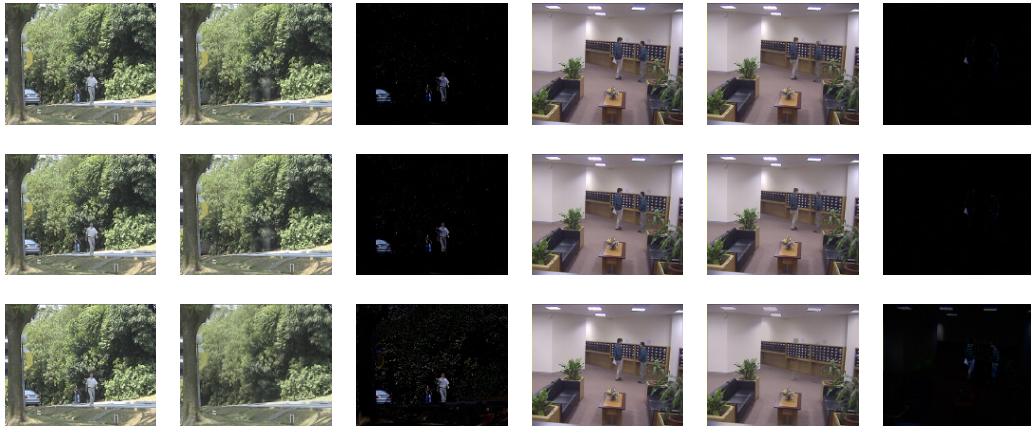
Figure 4: Background modeling results on campus and lobby dataset, where the first, second and third row corresponds to nuclear norm by IALM ( 1.62e+04 seconds/ 1.62e+04 seconds), partial singular value by PSSV ( 1.18+e04 seconds/ 1.18+e04 seconds) and spectral k-support norm by proposed I ( 6.33e+03 seconds/ 2.91+e03 seconds) correspondingly. The first three columns show original sample frame (file:trees1831) from campus and the corresponding background and foreground; the last three columns show sample frame (file:SwitchLight2457) from lobby and the corresponding background and foreground.
