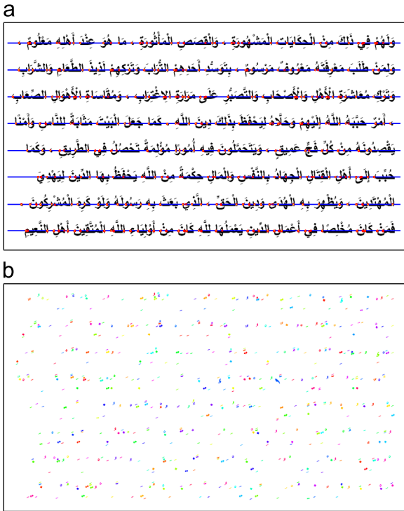
Fig. 6. Diacritics segmentation using flood-fill algorithm: (a) the input image with baselines (blue lines) and the flood-fill seeds shown in red circles while the actually used seeds are filled with yellow and (b) the resultant image. (For interpretation of the references to color in this figure caption, the reader is referred to the web version of this article.)
