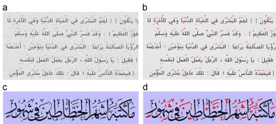
Fig. 16. Examples of testing our method with real images: (a) shows the noisy image written with Jaridah font, (b) shows the result of diacritics segmentation for the noisy image, (c) shows a colored low resolution (96 dpi) image written with Tholoth font, and (d) shows the result of diacritics segmentation for image (c). (For interpretation of the references to color in this figure caption, the reader is referred to the web version of this article.)
