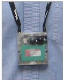
The v2.3 SenseCam shown close up and as typically worn by a user. The model pictured here has a clear plastic case that reveals some of the internal components.
