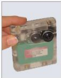
The v2.3 SenseCam shown close up and as typically worn by a user. The model pictured here has a clear plastic case that reveals some of the internal components.
