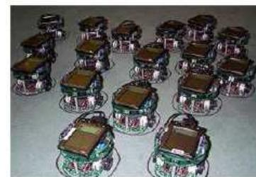
Fig. 2. A team of pherobots built for Darpa Software for Distributed Robotics program.
