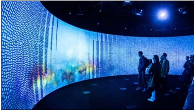
Fig. 2: A large cylindrical screen, four metres high and ten metres in diameter. A high performance computer graphics system drives six 3D-stereo video projectors, edge-blended to create a seamless three-dimensional panorama.
