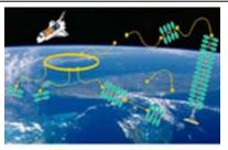
Schematic diagram of architecture of self-assembling solar power satellite. Seeker "whip" units, powered at both ends, listen for signals from subassemblies, find them, and pull them together.
