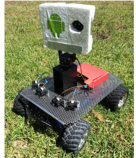
Figure 1. Android based robotic platform. The Android phone serves as the computing and sensing device. The IOIO provides an interface to add additional sensors, such as IR range finders. The base is installed on the chassis of a R/C truck. The robotic head is composed of a rectangular tube, two servos for the pan and tilt unit, and a phone holder made of foam. Adapted from [9].
