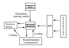
Fig. 1. Information system diagram. Extraction, transformation and loading process describe the interaction between the Gero and Koreisha databases.
