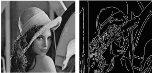
(a) The original image (b) Detecting result by wavelet Algorithm
