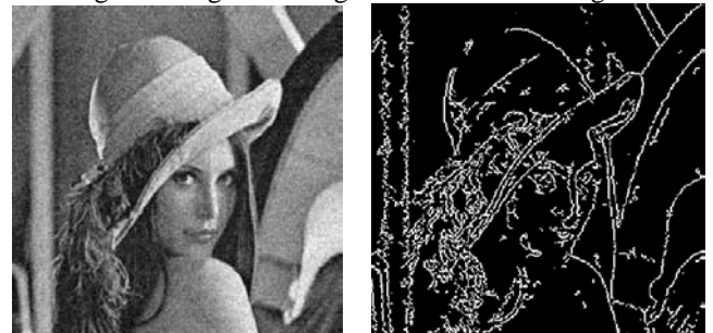
(a) The original noisy image (SNR=15.8dB) (b) Detecting result by wavelet Algorithm
