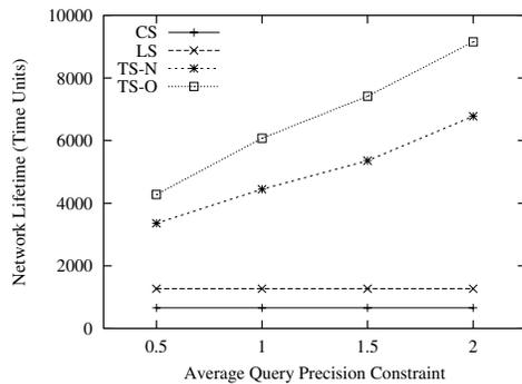
**Figure 10. Lifetime vs Precision Constraint (Temperature)**
