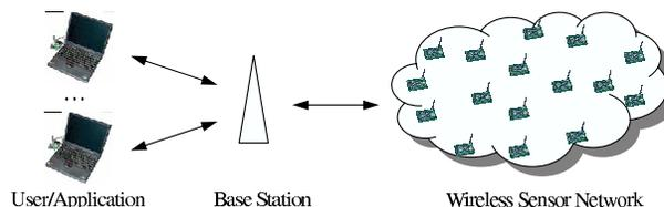
Figure 1. Sensor Network Architecture
