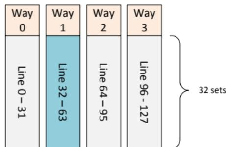
**Figure:** Fermi L1 Data Cache Structure
