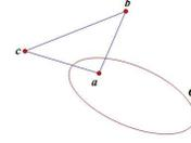
**Fig. 2.**  $\triangle abc$  is a self-polar triangle with respect to conic  $\mathbf{C}$  when polars of  $a$ ,  $b$  and  $c$  are lines  $bc$ ,  $ac$  and  $ab$ , respectively.
