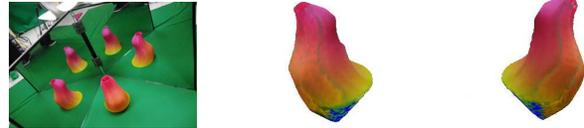
Fig. 9. The first image is a vase under a setting of two mirrors, while the second and third images are two views of the reconstructed vase by using our estimated intrinsic parameters.
