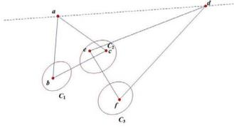
**Fig. 5.** Vanishing line  $ad$  of the support plane recovered from vertices of common self-polar triangle of circle images.
