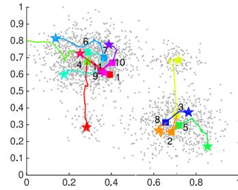
Fig. 11. Moving trajectory of seed points by SMCL on dataset *gaussian*. The square is the starting position and the star is the final position. The number indicates the appearing order of seed points.
