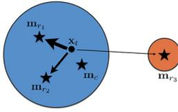
Fig. 4. Example of two imbalanced classes with four seed points.  $\mathbf{m}_c$  is the winner of  $\mathbf{x}_t$ .  $\mathbf{m}_{r_1}$ ,  $\mathbf{m}_{r_2}$ , and  $\mathbf{m}_{r_3}$  are three rivals. The majority cluster (in blue) is shared by three seed points and the minority cluster (in red) is represented by one seed point. The thickness of the arrow indicates the value of  $\beta_j$ .
