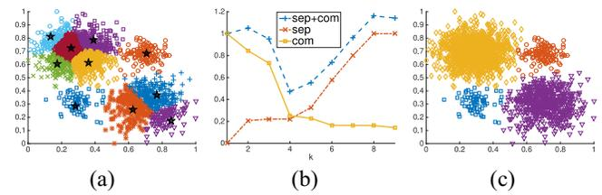
Fig. 7. Dataset *gaussian*. (a) Ten subclusters generated by PNS. (b) Global separability, global compactness, and their sum. (c) Clustering result by SMCL.
