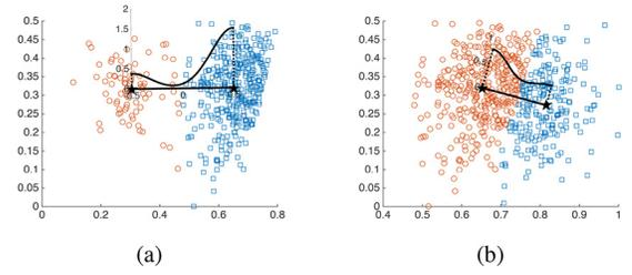
Fig. 6. Example of calculating separation measure by using 1-d Gaussian mixture probability density function. (a) Two subclusters belong to different clusters.  $s_{ij} = 13.37$ . (b) Two subclusters belong to the same cluster.  $s_{ij} = 2.86$ .
