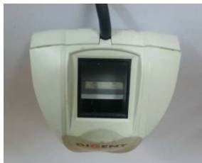
1. Optical sensor: 14.2mm×16mm
