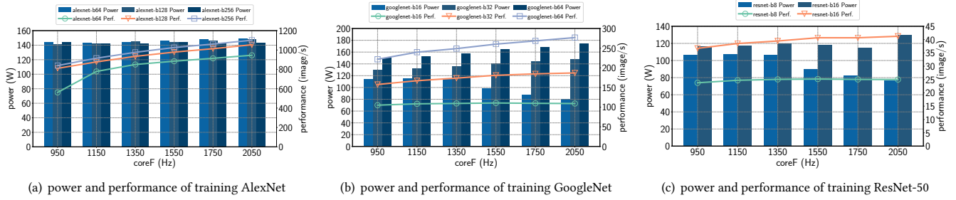
Figure 10: training using Winograd on GTX2080Ti with increase of core frequency
