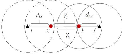
Fig. 2. Interference range between APs  $i$  and  $j$  [30].
