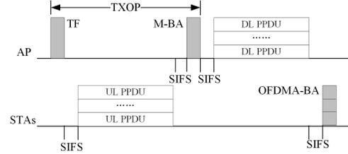
Fig. 1. Frame exchange procedure between an AP and its STAs [17].
