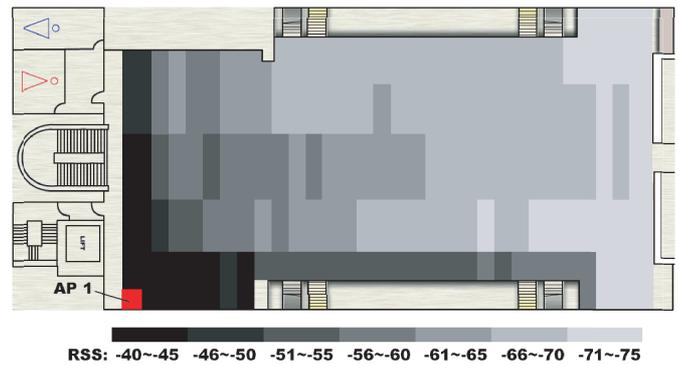
Figure 2. Signal Propagation of Access Point 1
