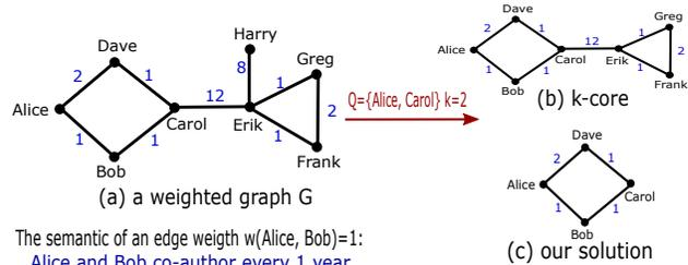
Fig. 1. An example intimate-core group query. (a) a given weighted graph  $G$ . (b) a  $k$ -core community retrieved by a general  $k$ -core algorithm without considering the weights in  $G$ . (c) a smaller community that has the minimum total weight retrieved by our approach. It can be confirmed that the community in (c) is semantically more intimate than the community in (b).
