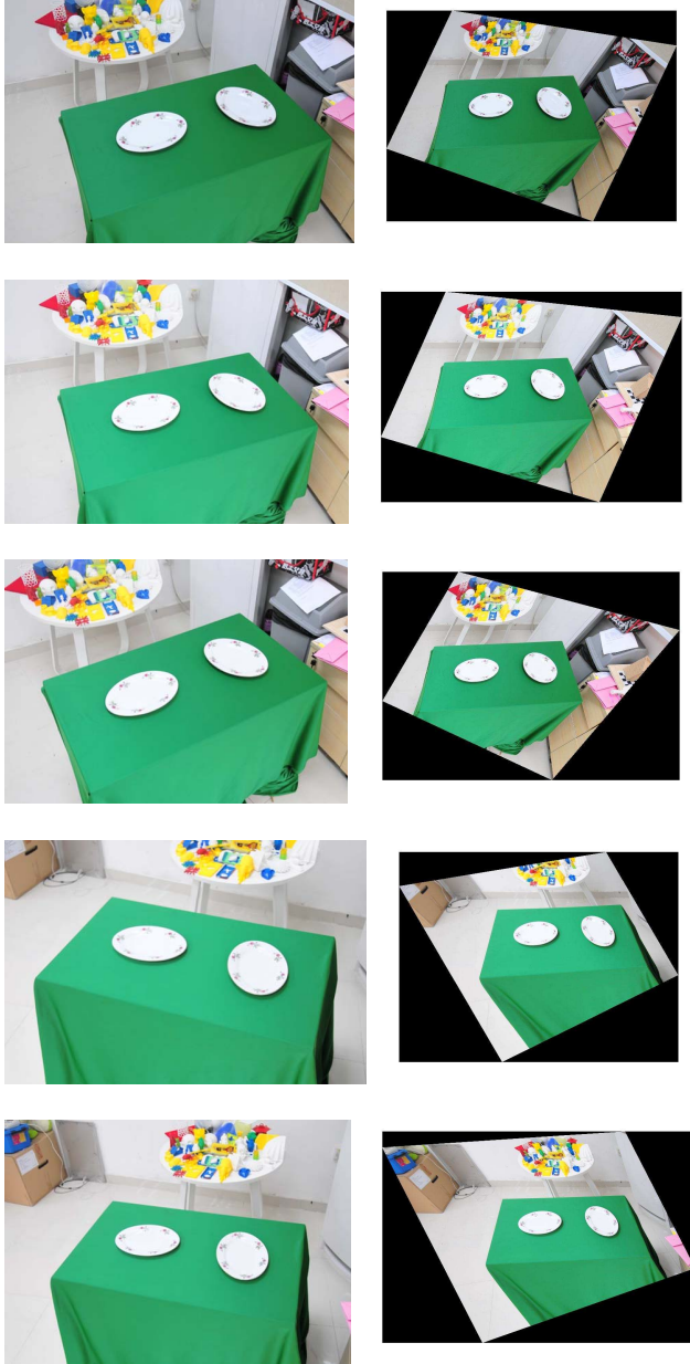
Figure 15. The left side are plate images taken from different view-points. The right side are images warped back to the reference view.
