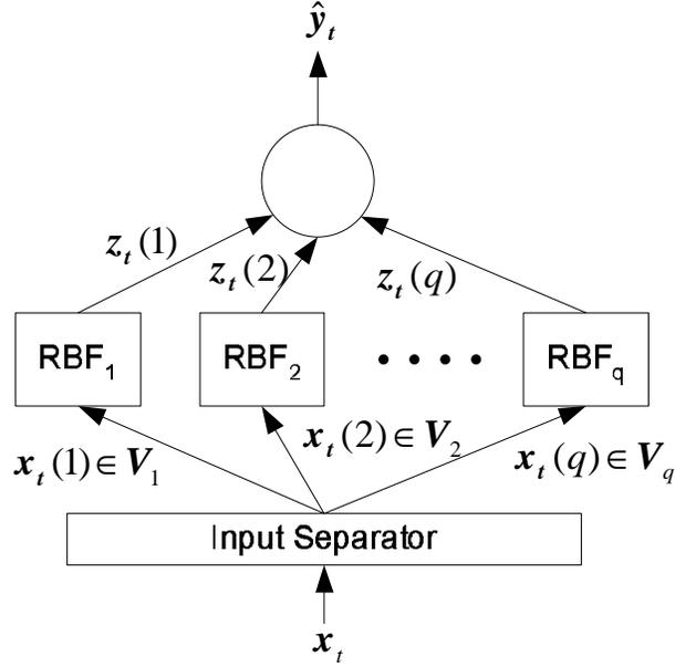
**Fig. 1.** The DCRBF network model.
